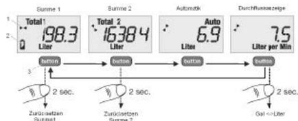
By shortly pushing the button you can switch between the different displays. The following can be shown on the display of the dial gauge:
